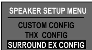
Selecting SURROUND EX from the SPEAKER SETUP menu (available in software Version 4) automatically sets the speaker selections for a THX SURROUND EX setup with two side and two rear speakers, and with all filters set to 80Hz. These settings are not adjustable.
