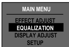
In the main menu, press SELECT to open the Equalization menu which contains Bass, Treble and Tilt controls, and a Loudness parameter.
