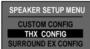
Selecting THX CONFIG from the SPEAKER SETUP menu automatically sets the speaker selections to the traditional configuration for THX listening. This configuration automatically sets REARS to NONE and all of the filters to 80Hz. These settings are not adjustable.
