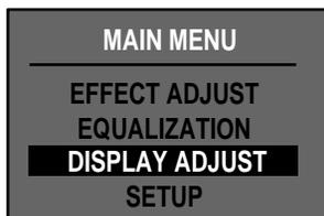
Depending on the location of the MC-1 in your room, you may need to adjust the brightness of the front panel display for optimum viewing. To adjust this display, press the ▲, ▼ or SELECT buttons on the Remote to enter the Main Menu. Press ▼ twice to select DISPLAY ADJUST.
